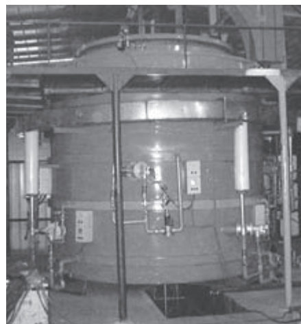
Direct heating of an annealing bell. Flue gases are recycled via the inductor.
