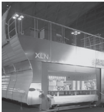
Roller hearth furnace
